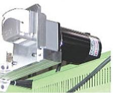
In addition to the varnish machine, an automatic neck combining glue coating system can be installed to complete varnish and neck combining gluecoating procedures at a time for reduction of time and cost.
