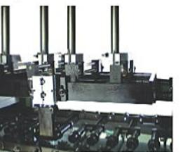
Automatic positioning and coating may place varnish unto the same location of the rotor precisely for uniformity.
